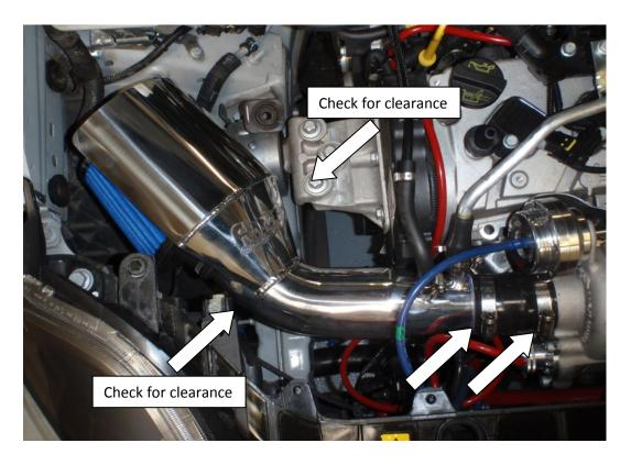
6. Using jubilee clips supplied in the kit tighten the silicon hose holding the induction pipe in the correct position. The breather pipe may need to be slightly bent to align with the new induction kit, Tighten the jubilee clips and your installation is complete!
