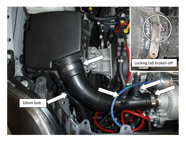
4. Remove the pin in the turbo housing to allow the silicon hose to fully fit.
